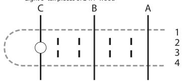
DETAIL: Plastic bin sits on line C. The eight wooden blocks, standing on end, will be placed in two lines (4 per line),  $6-\frac{1}{2}$ " apart (width). Starting out from line B, the second and third blocks will be  $3-\frac{1}{2}$ " from line B. From the second to first and third to fourth, the length will be  $6-\frac{1}{2}$ " between blocks.
