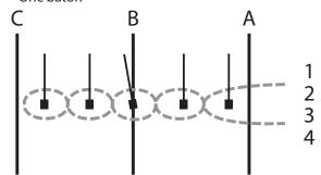
DETAIL: A bending pole is a plastic pole in a metal, plastic, concrete or rubber cone base (total height 4'6"). The baton is 10"-12" long, 1" in diameter.
